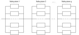
Figure 4: A series-parallel system
